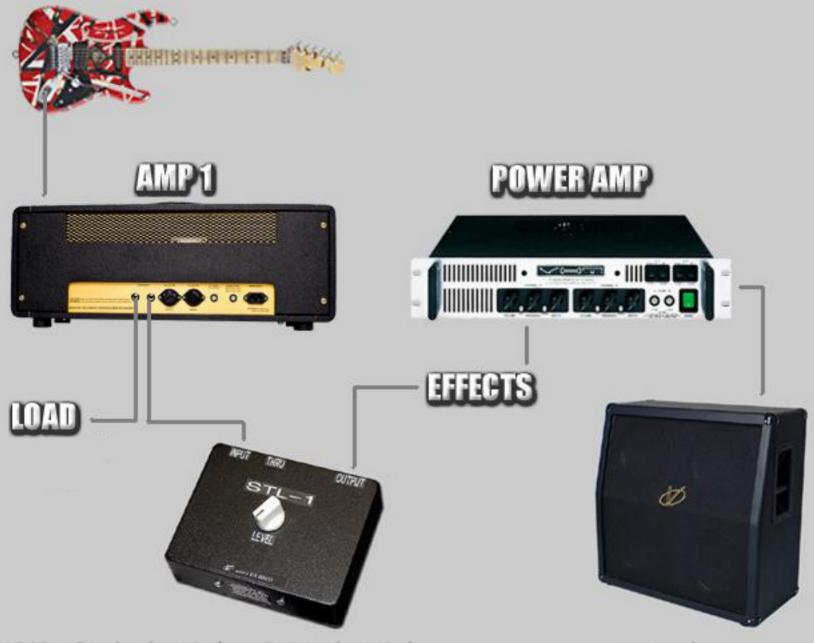
LOAD = Speaker (reactive) or Resistor (resistive)
