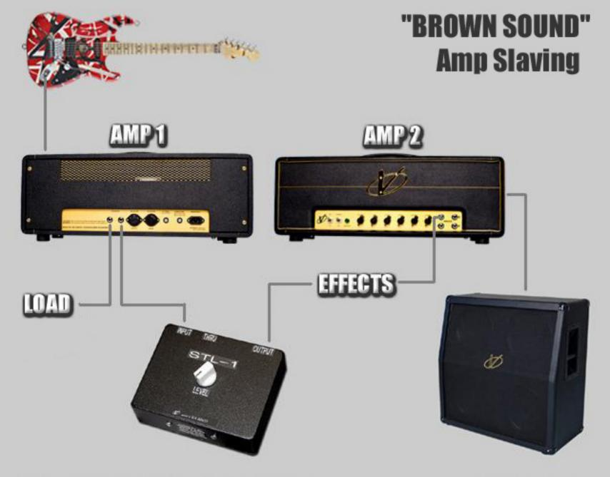
LOAD = Speaker (reactive) or Resistor (resistive)
