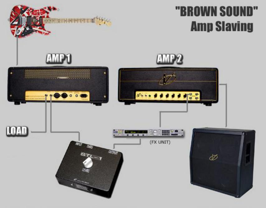
LOAD = Speaker (reactive) or Resistor (resistive)
