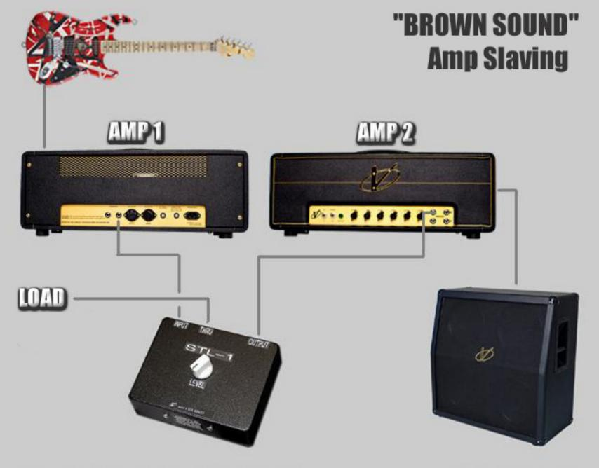
LOAD = Speaker (reactive) or Resistor (resistive)
